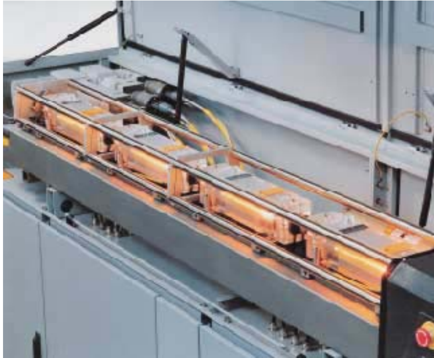
Nd:YAG laser with 4 cavities and 2 kW power
