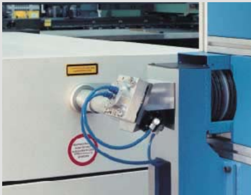
Phase shifter: the principle is shown above. Below the circular polarizer of a CO 2 laser.
