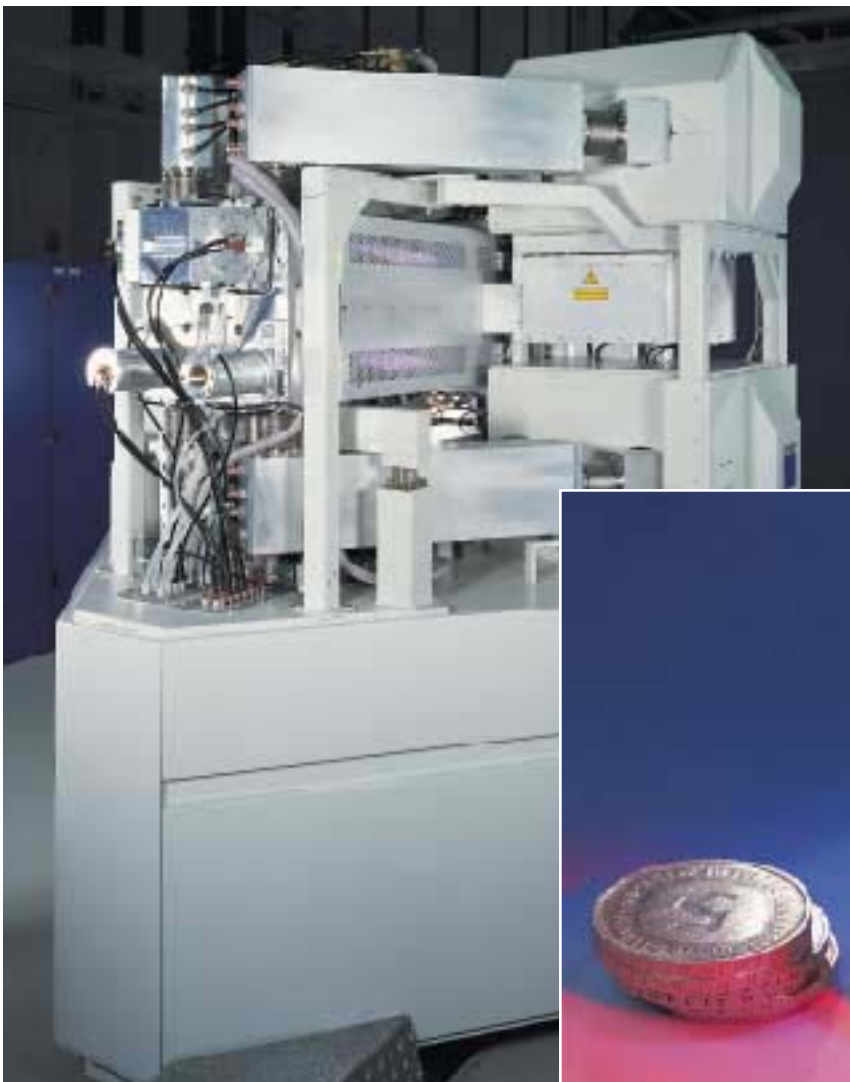
Large and small high-powered lasers: CO 2 laser (30 kW) and diode laser (200 W)
